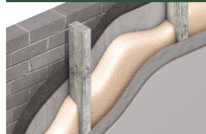
✓ Timber frame walls
